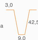
$\emptyset 5 \text{ mm c. } 20 \text{ cm } 130:20 = 6 \text{ estribos}$
